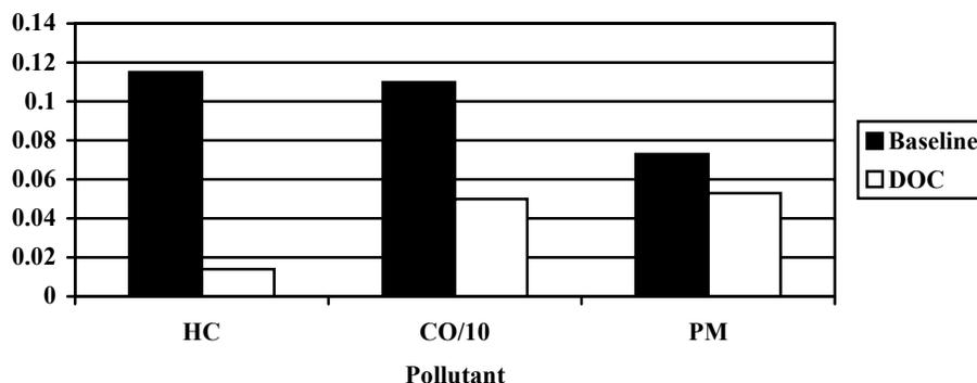
Like catalyst-based DPFs, oxidation catalysts are effective in controlling toxic HC emissions. The control capabilities of two DOCs were evaluated for 18 distinct PAHs (Reference 1). Reductions in excess of 50 percent are readily achieved with reductions approaching 70 percent possible. Similar or better results can be expected on steady-state test cycles for the reasons mentioned above for catalyst-based DPFs.
