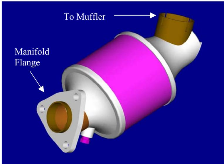
Also, exhaust emission control technology can be designed and integrated on to vehicles to address special operating concerns and environments. For example, where equipment is used in explosive operating environments, such as underground coal mines, emission control technology has been designed to meet special surface temperature requirements. Also, exhaust emission control technologies can and have been installed on vehicles so as not to impair operator visibility.
